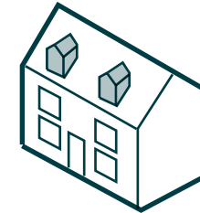
Loft conversion incorporating gable dormer which are aligned to windows.
