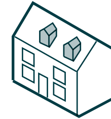
Loft conversion incorporating gable dormers which are not aligned to windows.
